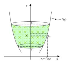
$$S = 2\pi \int_{a}^{b} x \sqrt{\left(\frac{dx}{dy}\right)^{2} + 1} \cdot dy$$
