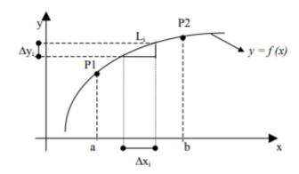
$$\begin{split} L_i^2 &= \Delta y_i^2 + \Delta x_i^2 \\ L_i &= \sqrt{\Delta y_i^2 + \Delta x_i^2} \\ L_i &= \sqrt{\left(\frac{\Delta y_i}{\Delta x_i}\right)^2 + I \cdot \Delta x_i} \end{split}$$
