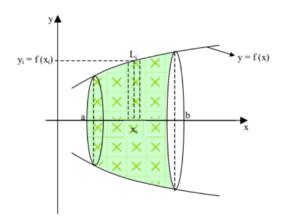
$$\begin{split} Si &= 2\pi f(x_i) L_i \\ S_i &= 2\pi f(x_i) \sqrt{\left(\frac{\Delta y_i}{\Delta x_i}\right)^2 + I \cdot \Delta x_i} \\ S &= \lim_{n \to \infty} \sum_{i=1}^n 2\pi f(x_i) \sqrt{\left(\frac{\Delta y_i}{\Delta x_i}\right)^2 + I \cdot \Delta dx} \\ S &= \int_b^a 2\pi f(x) \sqrt{\left(\frac{dy}{dx}\right)^2 + I \cdot dx} \text{ ou } S = 2\pi \int_a^b y \sqrt{\left(f'(x)\right)^2 + I \cdot dx} \quad \to \text{ Superficie gerada pela revolução} \end{split}$$
